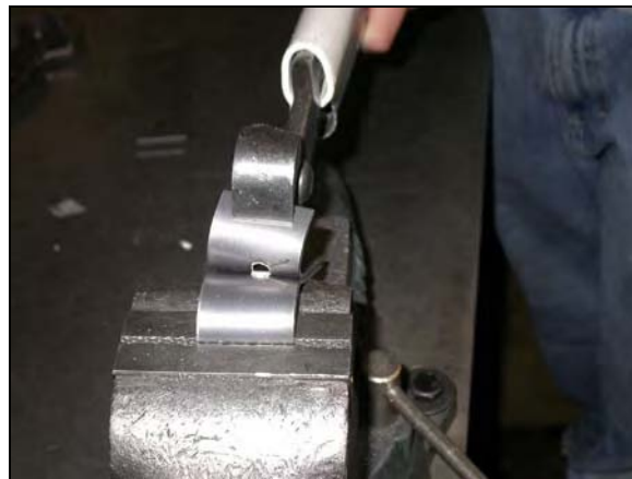
Figure D3 Peeling has initiated a button pull from one of the sheets.
