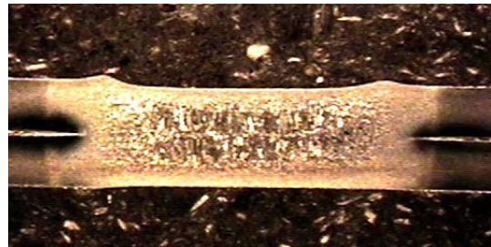
Figure F7 Photograph of cross section of same weld (DP-600), 0.7 mm thick
