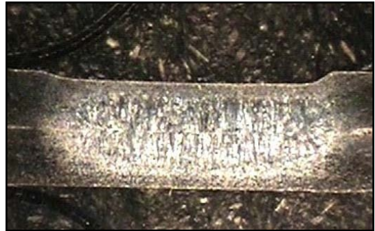
Figure F9 Cross section of acceptable weld in low carbon steel
