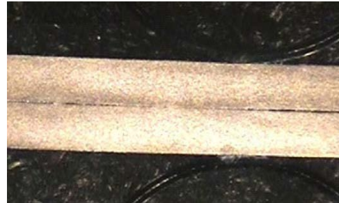
Figure F11 Cross section of stick weld in DP-600
