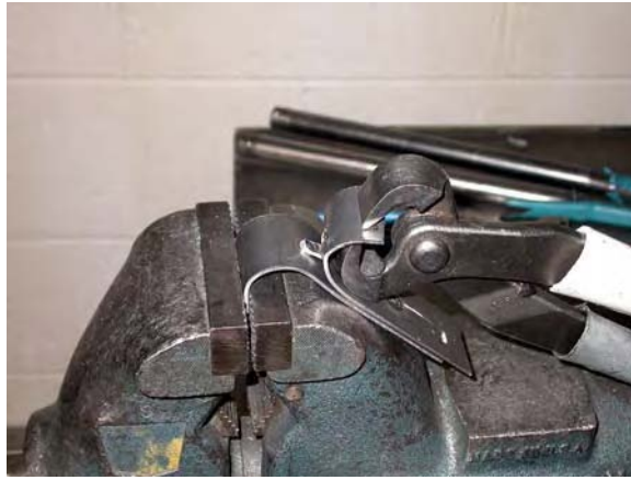
Figure D4 Peel testing producing metal “teardrop”
