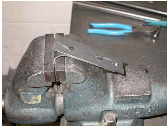
Figure D2 Sample bent for application of peeling tool
