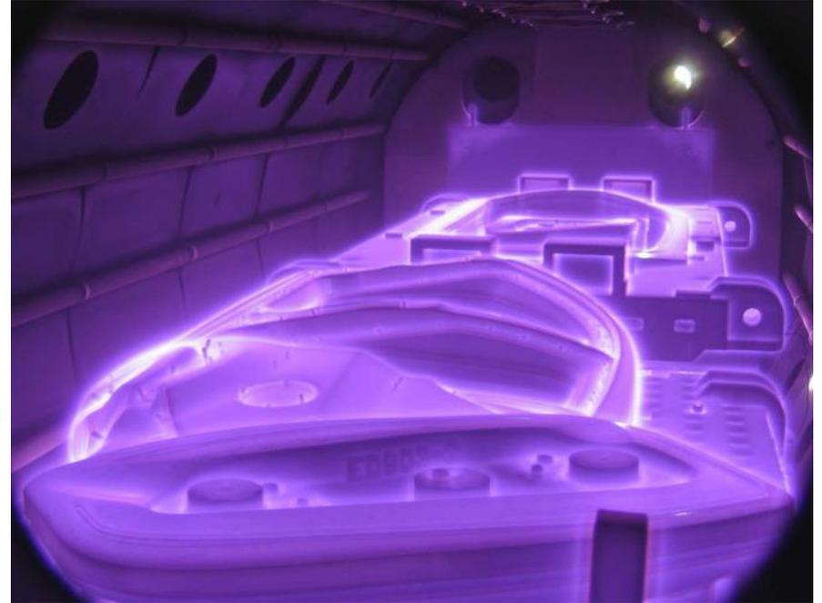
Chrome plating and nitriding have been used to improve the durability and wear resistance of stamping dies.
