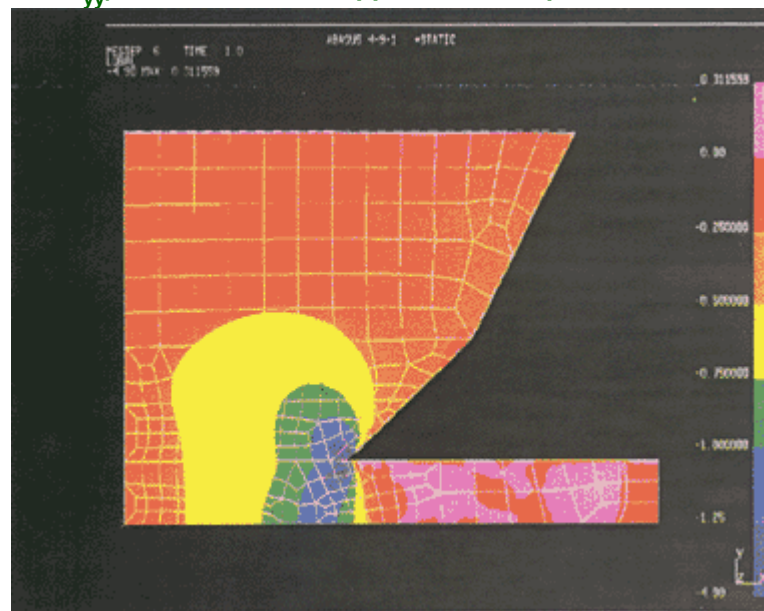
Figure 5. Pressure ( \sigma_{yy} ) distribution after application of squeeze force.
